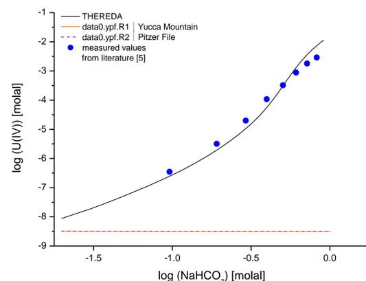
Fig. 2: Solubility of U(OH)<sub>4</sub>(am) in NaHCO<sub>3</sub> solution at T = 25 °C.
