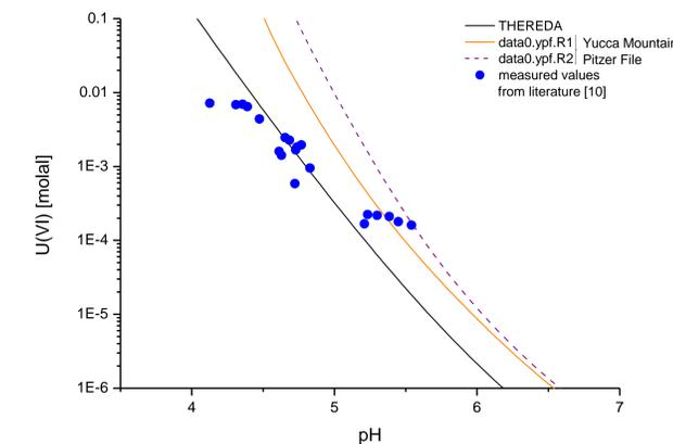
Fig. 5: Solubility of Becquerelite in 1 m CaCl<sub>2</sub> solution at T = 25 °C.
