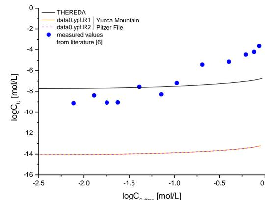
Fig. 3: Solubility of U(OH)<sub>4</sub>(am) in Na<sub>2</sub>SO<sub>4</sub> solution at T = 25 °C and log(C<sub>H+</sub>) = -4.5.
