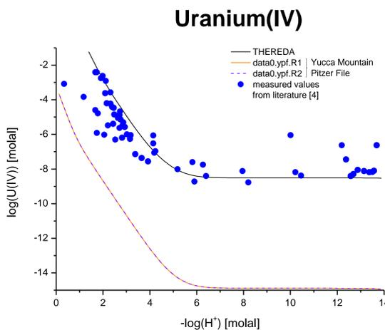
Fig. 1: Solubility of U(OH)<sub>4</sub>(am) in 1 m NaCl solution at T = 25 °C.
