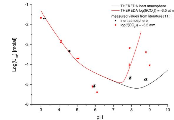
Fig. 6: Solubility of Soddyite in 0.1 M NaClO<sub>4</sub> solution at T = 25 °C.
